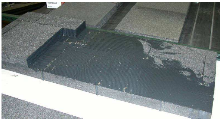
Figure 8. Coal-based carbon foam bonding adhesive.
