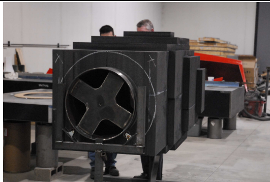
Figure 18. Installation of inside tool holding fixture.
