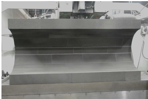
Figure 17. Coal-based carbon foam inside mandrel rough machining.
