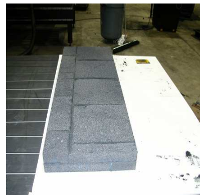
Figure 9. Bonded coal-based carbon foam billets.
