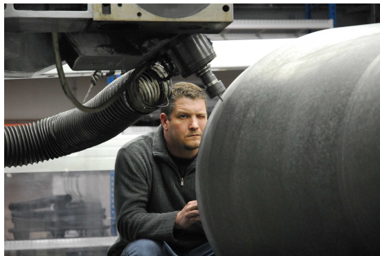
Figure 20. Machining of chopped carbon surface.
