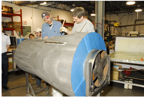
Figure 19. Installation of thermocouples and chopped carbon surface.
