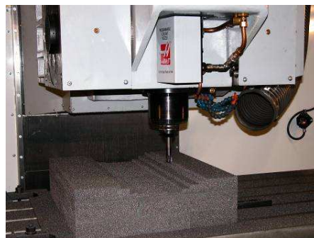
Figure 10. Coal-based carbon foam rough machining.
