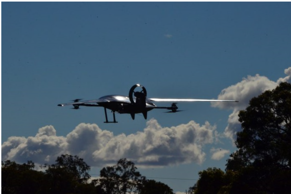
InnovaeroFOX at 30 per cent scale in VTOL mode undergoing hover testing in November 2020.
