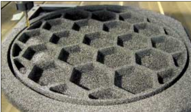
Fig. 5 — Machinability of carbon foams is shown on this mirror backing.
