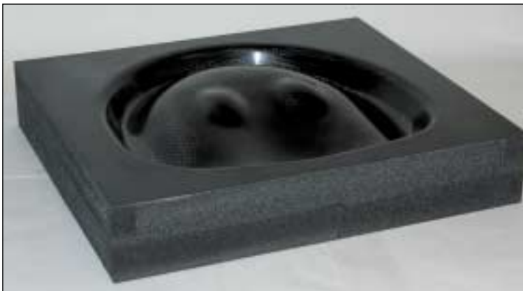
Fig. 4 — CFoam composite tool with low coefficient of thermal expansion.
