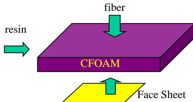
**Figure 3(a).** Schematic of combined adhesion and infiltration process.
