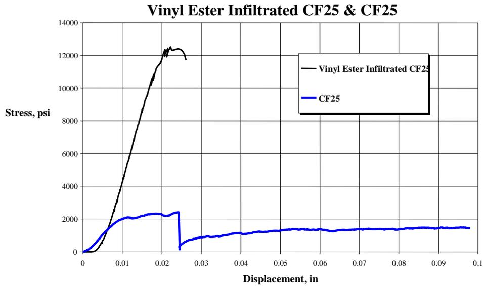
**Figure 5(b).** Compression test of CF25 infiltrated with vinyl ester resin.
