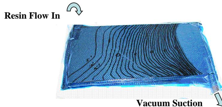
**Figure 2.** Infiltration apparatus.
