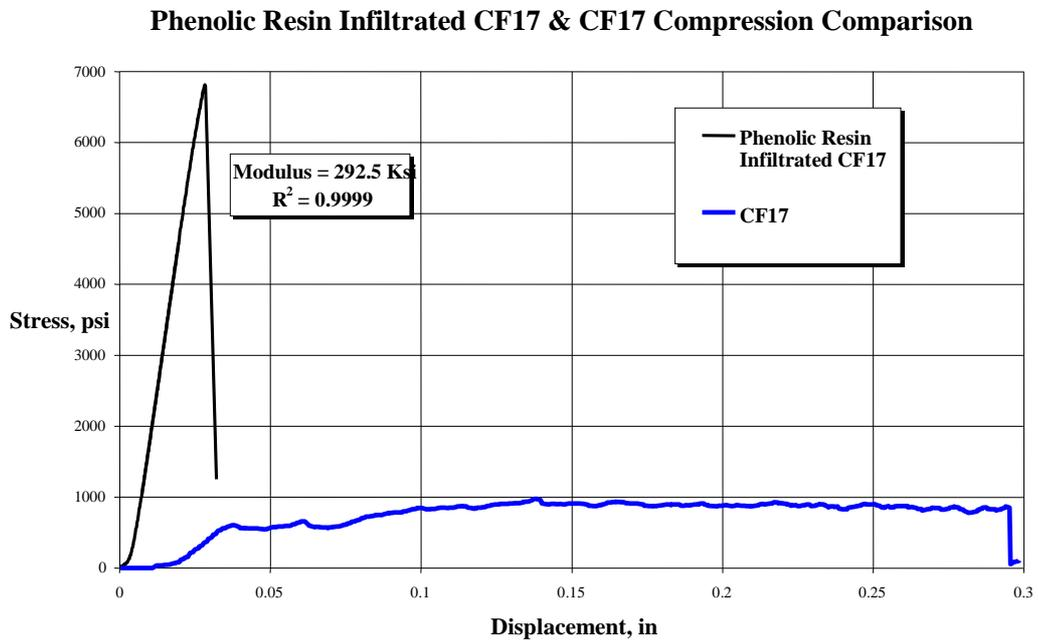
**Figure 5(a).** Compression test of CF17 infiltrated with phenolic resin.
