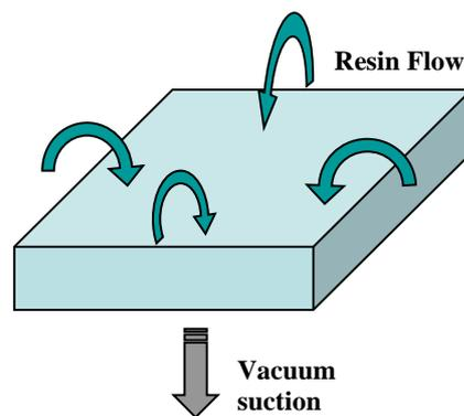
**Figure 1.** Schematic of resin infiltration through a CFOAM block.
