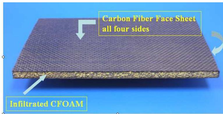
**Figure 3(b).** Finished Part by combined infiltration and adhesion process (1/4" CF17 panel infiltrated with phenolic resin and bonded with carbon fiber sheets at all four sides).
