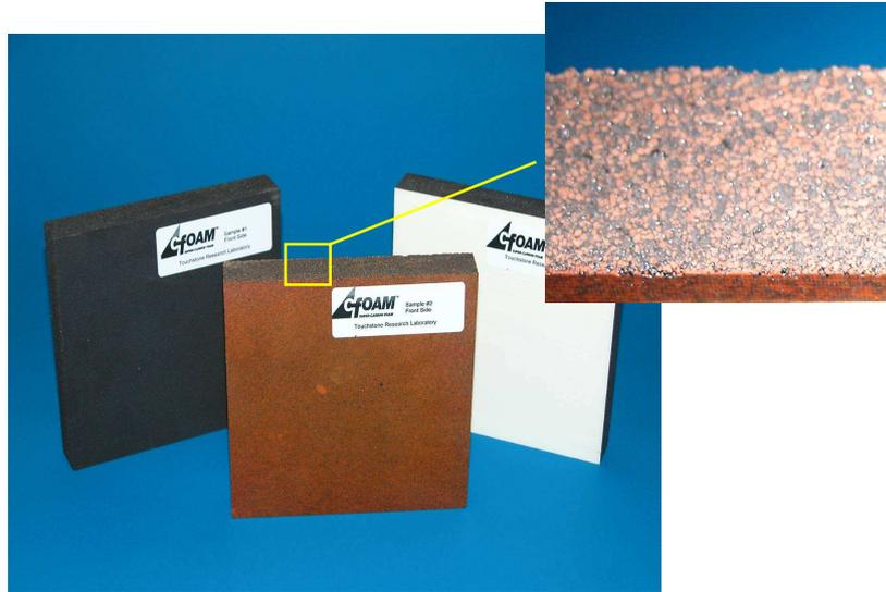
**Figure 4.** CF17 infiltrated with phenolic resin.
