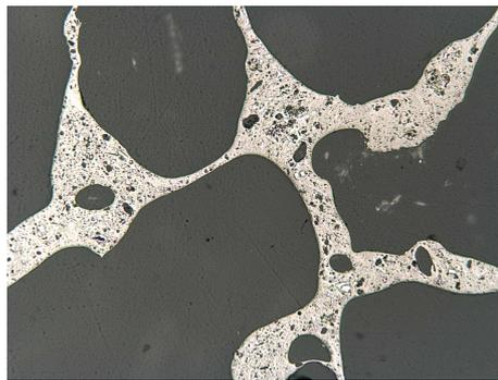
**Figure 6.** 100X microscopic image of CF17 infiltrated with epoxy resin.
