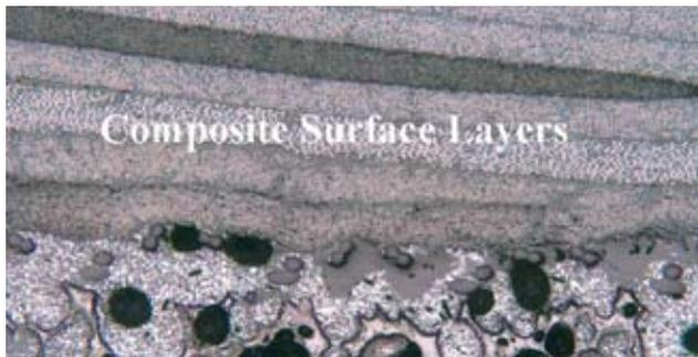
Figure 4. Coal-based carbon foam SEM image.
