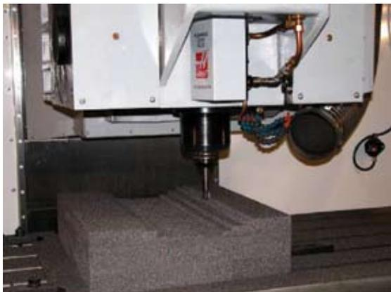
Figure 10. Coal-based carbon foam rough machining.
