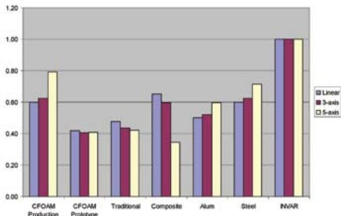
Figure 5. Graph of comparative tooling cost relative to Invar 36.
