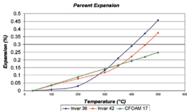
Figure 3. Coal-based carbon foam CTE vs. Invar 36 & 42.
