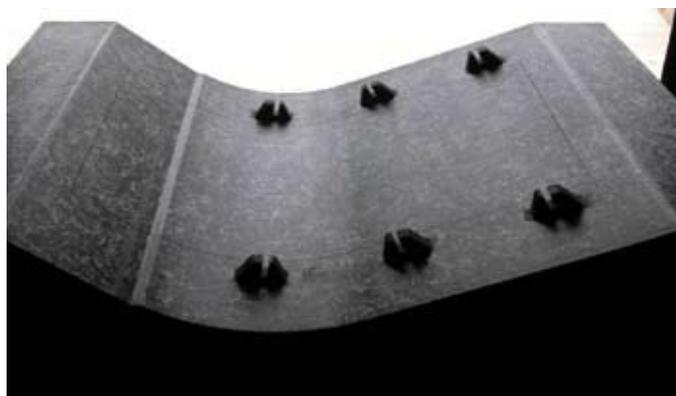
Figure 1. Coal-based carbon foam tooling.
