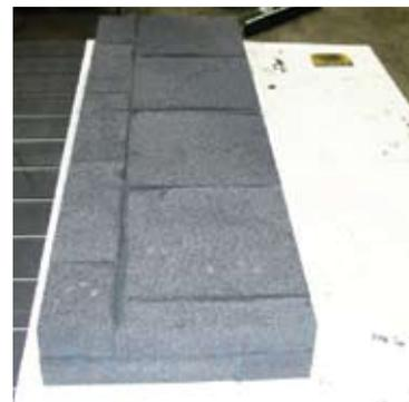
Figure 9. Bonded coal-based carbon foam billets.
