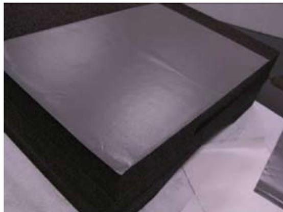
Figure 11. Prepreg applied to bottom.
