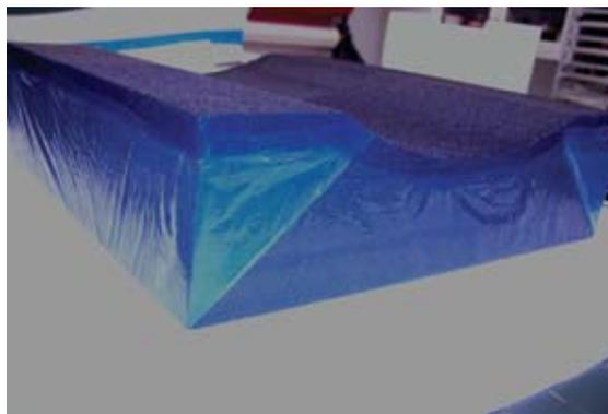
Figure 12. Prepreg applied to the sides.
