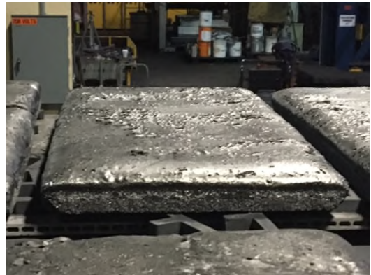
Untrimmed calcined billet of PFOAM™
